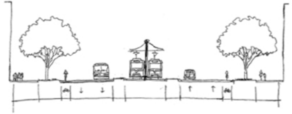
A cross-section of North Temple after Airport Light Rail construction shows a complete street, with space for pedestrians, bicyclists, cars and transit.
